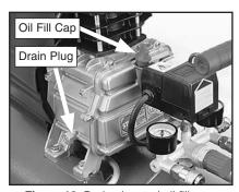
Figure 18. Drain plug and oil fill cap.
